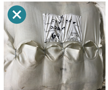
Excessive tension when closing off bale creating a wrinkled label.
