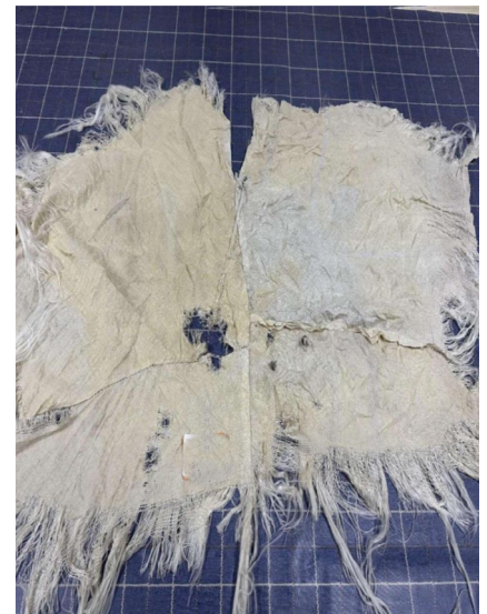
Pack material has broken down after scouring resulting in batch contamination.
