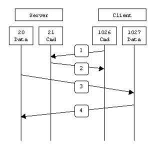
In step 1, the client's command port contacts the server's command port and sends the command PORT 1027. The server then sends an ACK back to the client's command port in step 2. In step 3 the server initiates a connection on its local data port to the data port the client specified earlier. Finally, the client sends an ACK back as shown in step 4.
