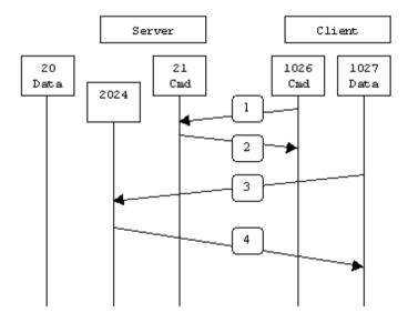
In step 1, the client contacts the server on the command port and issues the PASV command. The server then replies in step 2 with PORT 2024, telling the client which port it is listening to for the data connection. In step 3 the client then initiates the data connection from its data port to the specified server data port. Finally, the server sends back an ACK in step 4 to the client's data port.
