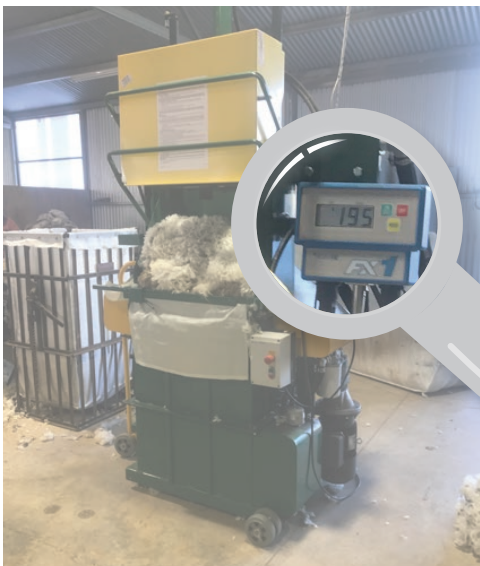
Inaccurate scales on the grower's wool press may be a cause of overweight bales.
