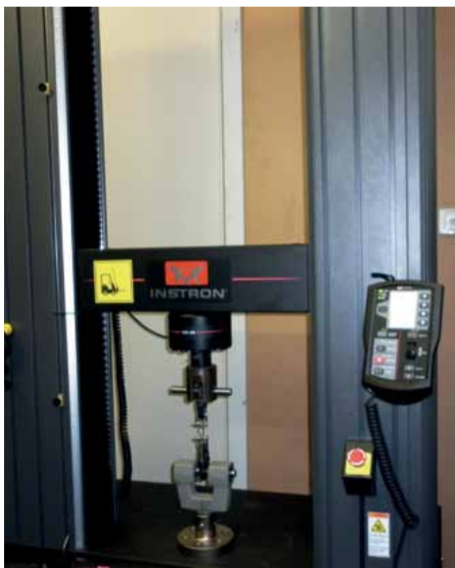
Instron Load Testing (a) Instron measurement (b) Instron output and (c) Fasteners after Load Testing
