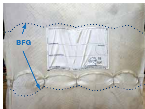
Bale Fastening Guide on all 4 Flaps. Fasteners must reach the BFG.
